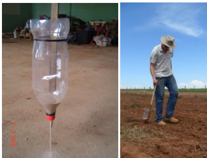
Fig. 2. Apparatus developed for sowing amaranth using pet bottle in Lucas do Rio Verde, Mato Grosso, Brazil
