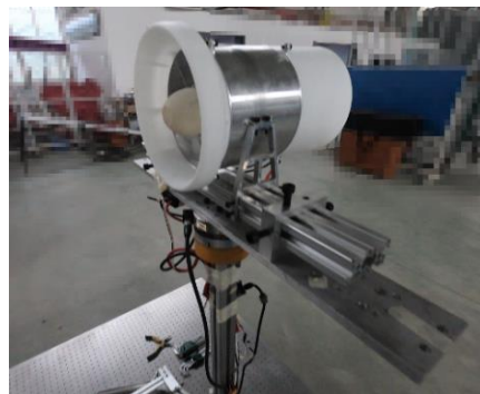
Figure 3. Experimental site and connection mode of the 150 ducted fan.
