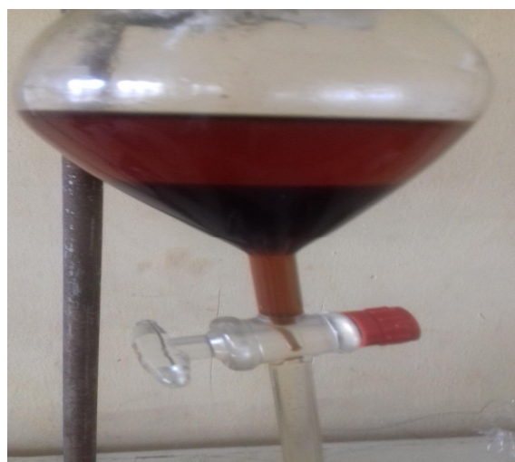
Fig. 3. Biodiesel-glycerin separation from palm oil sludge
