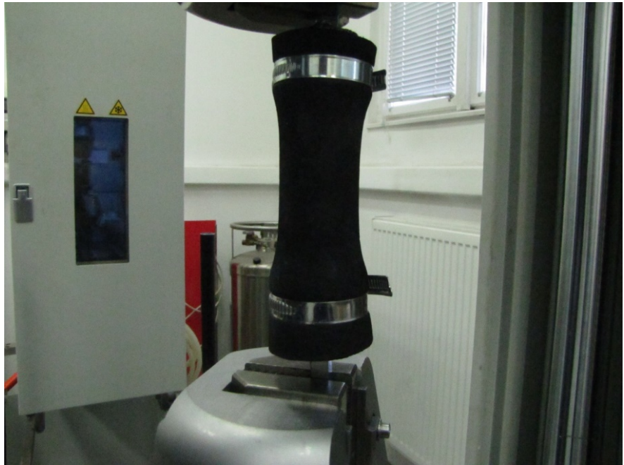
Figure 20. Hose piece subjected to tensile load at a displacement of 25 mm.
