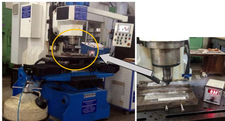
Figure 1. Close up view of sample prior to processing and applied cryogenic coolant.
