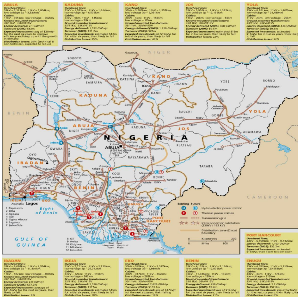
Fig. 4. National electricity transmission grid of Nigeria [49]
