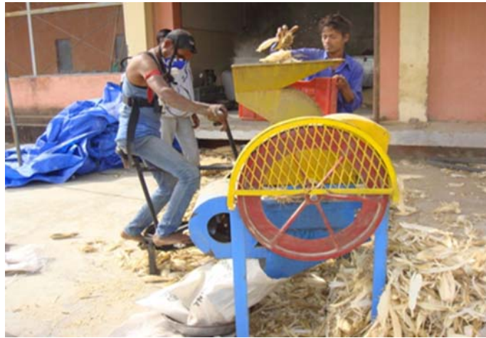
Fig. 1. Operational view of Pedal Operated Maize Dehusker Sheller
