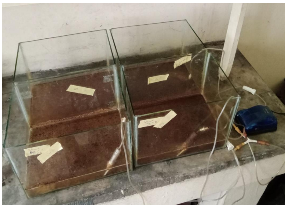
Plate 1. Air bubbling into the simulated crude-oil polluted water body with the aid of aquarium air pump, drip-set tubing, and Y-tubes. [The control setup is the glass trough at the left-back, setup A is at the right-back, setup B at the front-right, and setup C at the front-left]
