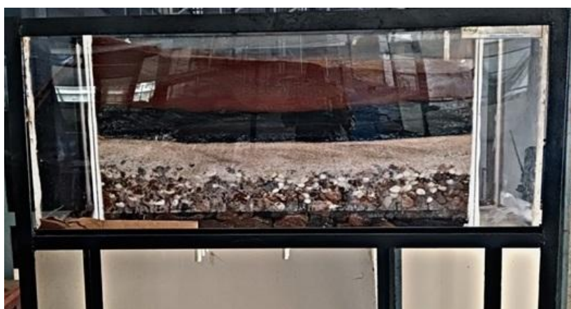
Fig. 7. Constructed wetland in laboratory scale after arranging the media
