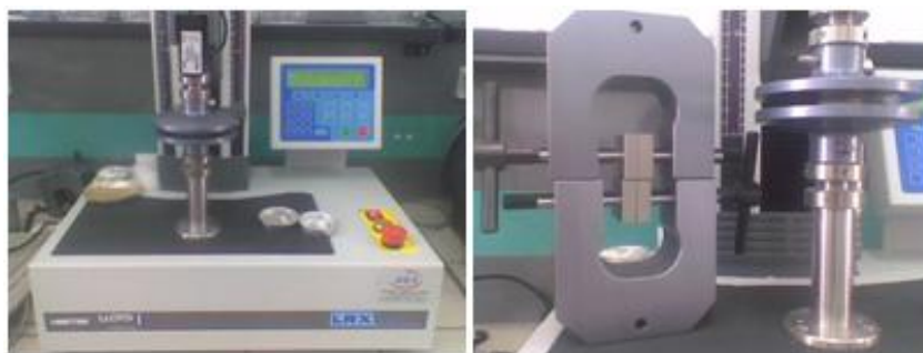
Fig. 3. Traction compression machine (LRX plus) with console (Ref. No. 01/2962)
