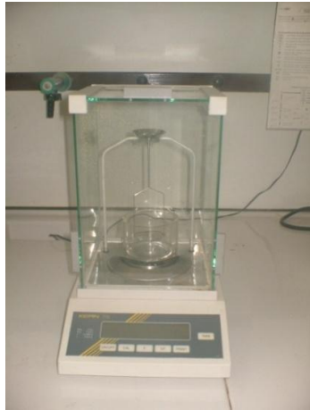
Fig. 2. Experimental apparatus for the apparent density determination installed on a precision balance
