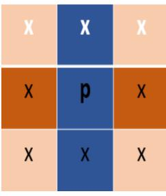
Fig. 3. 8-Connected pixel
