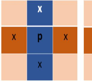
Fig. 2. 4-Connected pixel
